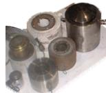
Various compression loadcells used for platform weighing jobs
